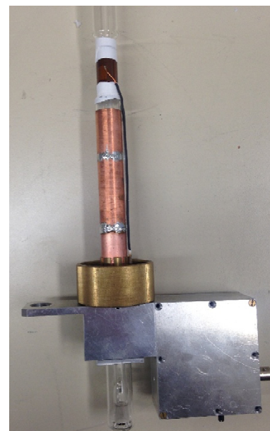
Figure 1. The high-temperature NMR probe used for the FFC measurements on Stellar Spinmaster FFC2000 relaxometer
