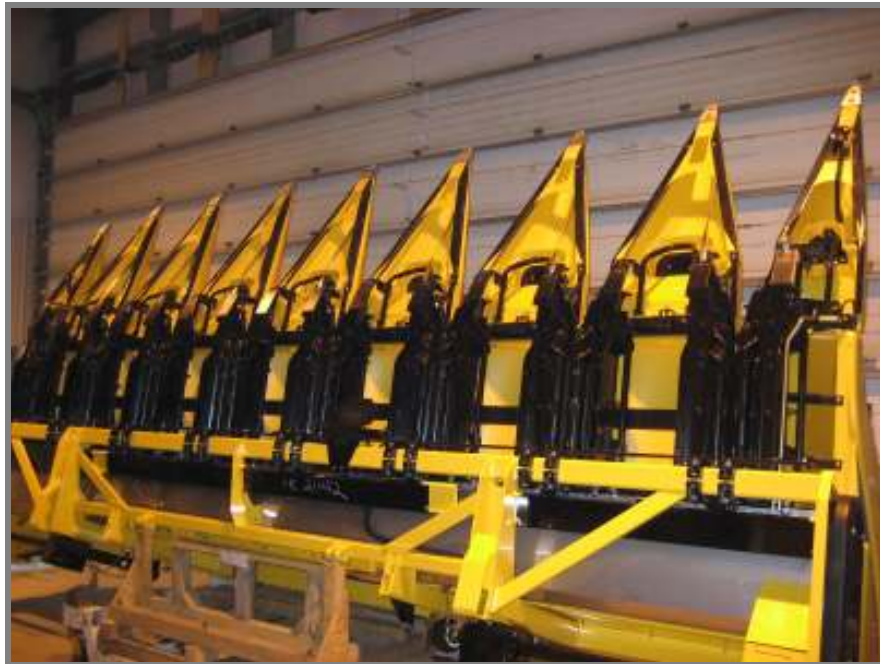
FIG 3.1A: A COMBINE WITH 8 ROW UNITS
