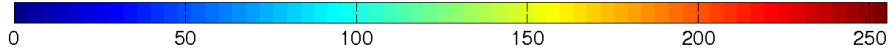
Figure 4.2: The colour bar used in the images of this section. Pixel intensity is mapped to a colour between light blue and dark red.
