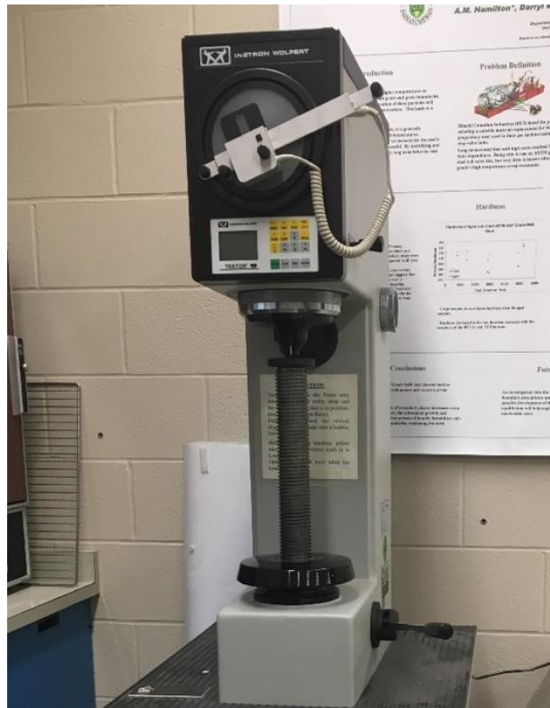
Figure 3.15. The Rockwell C hardness tester used in this work
