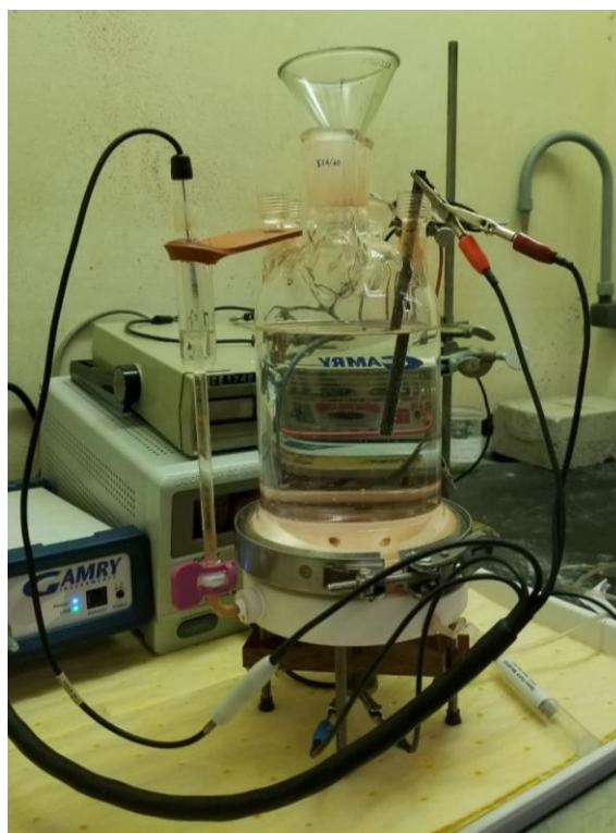
Figure 3.19. The electrochemical cell setup connected to the potentiostat used in this work
