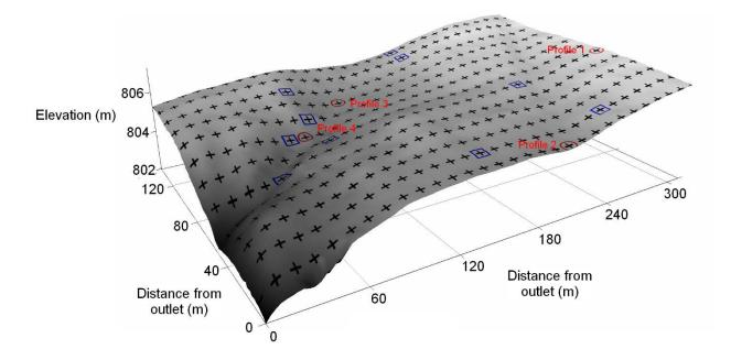
**Figure 4.1** Digital elevation model of the surface topography of Hillslope 2, with vertical exaggeration. Also shown: 10 x 10 m measurement grid (plus signs), locations of the four soil moisture and soil temperature profiles (red circles), and locations of the 11 snowmelt lysimeters (blue squares).
