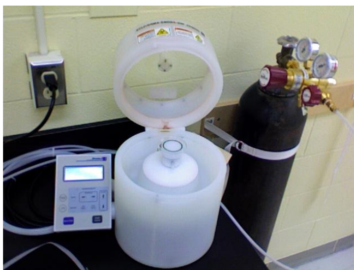
Figure 4.1. Image of spin coater equipment with nitrogen source attached.
