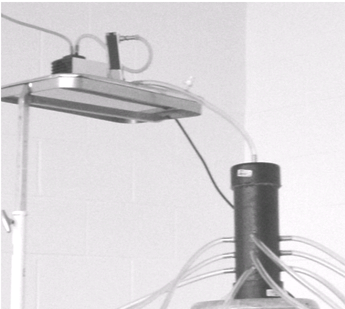
Figure 2-6. Pictured are 9 of the 12 individual holding chambers exhaust gas lines emptying into the black PVC filter housing unit (bottom). An exhaust line running to the bottom of the exhaust flow meter is attached to the 0.2 CFM vacuum pump (001-78164-00, Cole Parmer Canada Inc., Anjou, PC, Canada) that exits to a HEPA filtration system.
