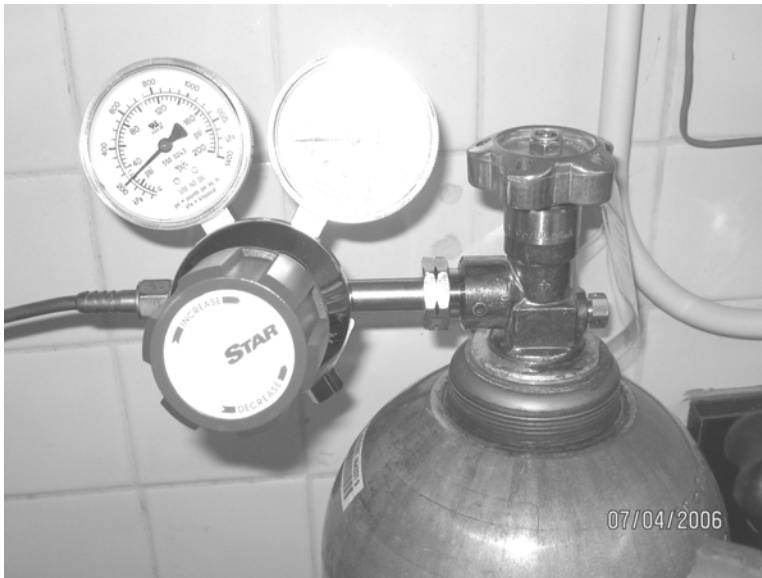
Figure 2-1 Re 212 dual stage chrome-plated forged brass body five port configuration, 316 L stainless steel diaphragm regulator with a compressed gas association (CGA) 590 connection supplied by Praxair (PRX 212-3301-75-000, Praxair, Saskatoon, SK, Canada) attached to ¼” compression X 3/8” hose barb brass fittings for control of the benzene toluene gas mixture release.
