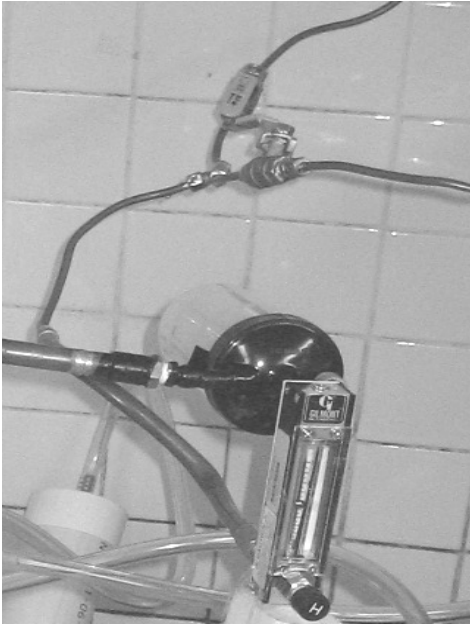
Figure 2-3 Inlet port of the 316 stainless steel 65-mm direct reading 0-10 LPM Gilmont flow meter solid arrow (C-32014-17, Cole Parmer Canada Inc, Anjou, PC, Canada) attached to the gas feed system by 1/2" Cu soft pipe by a 1/8" FIP and at the top to the 350 cc Salter 7600 bubble humidifier hollow arrow (Medigas Saskatoon, SK, Canada) wing nut all exiting to the 1/2" hard Cu pipe leading to the animal chambers on the hexagon bases.
