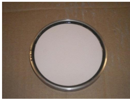
b) Front view of the new 15-bar plate mounted on a steel ring in the Engineering Shops, U of S
