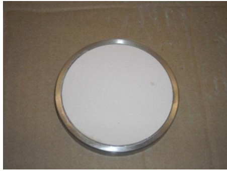
a) Back view of the new 15-bar plate mounted on a steel ring in the Engineering Shops, U of S
