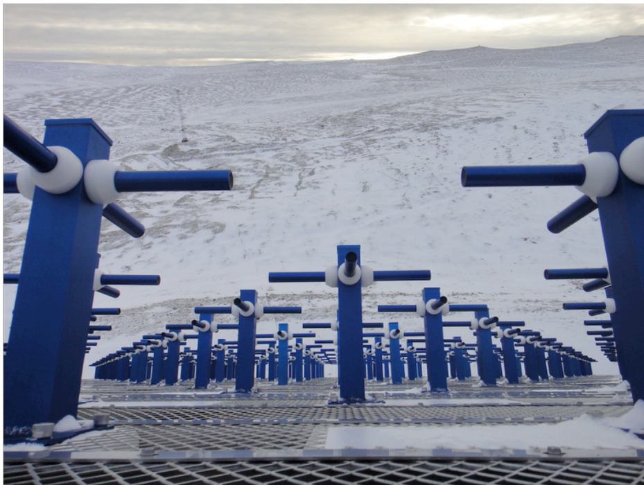
Figure 2.5: A closer view of the RISR-N face, showing some of the many thousands of antennas. Photo courtesy of C. Heinselmann.
