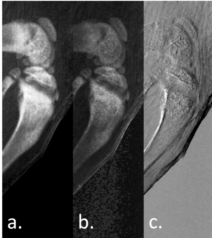
Figure 29 Sagittal DEI images the rat tibia – fibula 1A specimen acquired with the Nesch laboratory based system. Figure a is an image acquired at the analyzer peak, figure b is an extinction image and figure c is a refraction image.
