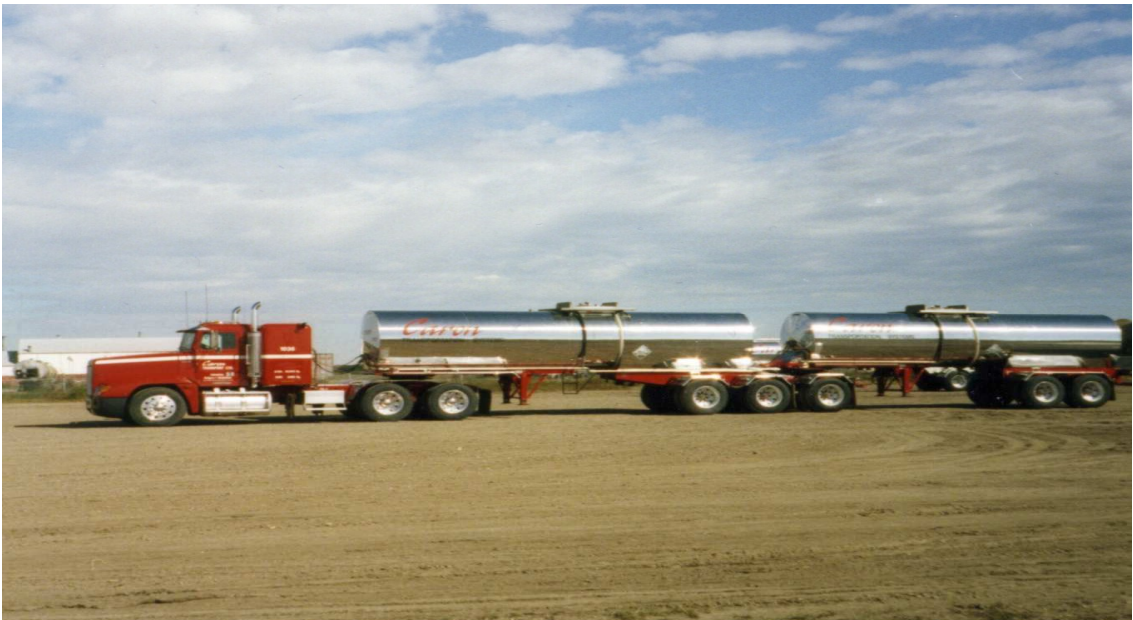
Figure 2.4: Eight - Axle B-Train Double
