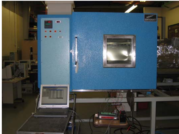
Figure A.2 Calibration setup of temperature sensors
