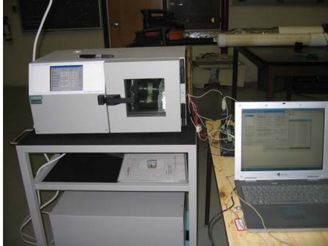
Figure A.4 Calibration setup of relative humidity sensors
