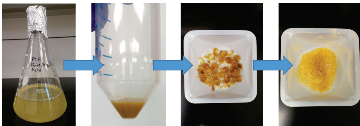
Figure 4-1 Dried FTI14 preparation procedure: culture growth, centrifugation, oven-drying, and grinding to fine powder.
