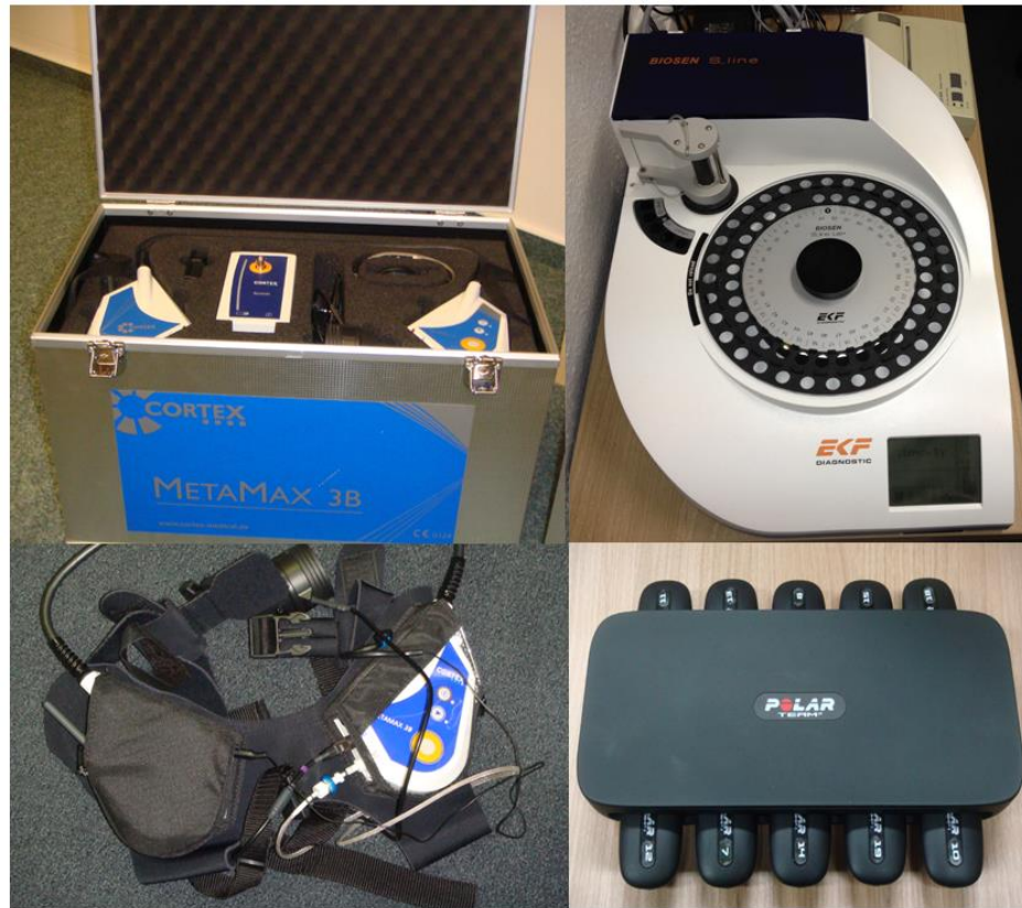
Figure 2: Portable metabolic, heart rate and blood lactate measuring equipment.
