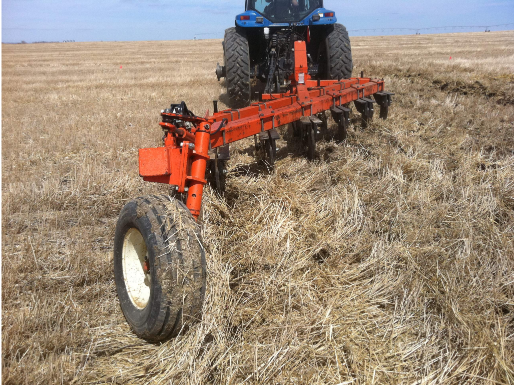
Fig. A4. Paraplow in ground tilling 45 cm deep
