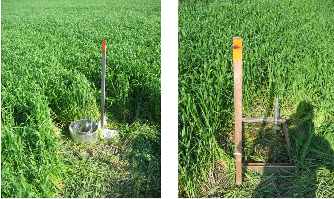
Fig. 3.3. Double ring infiltrimeter apparatus (left) & large ring infiltrimeter apparatus (right) in field – Summer 2010.
