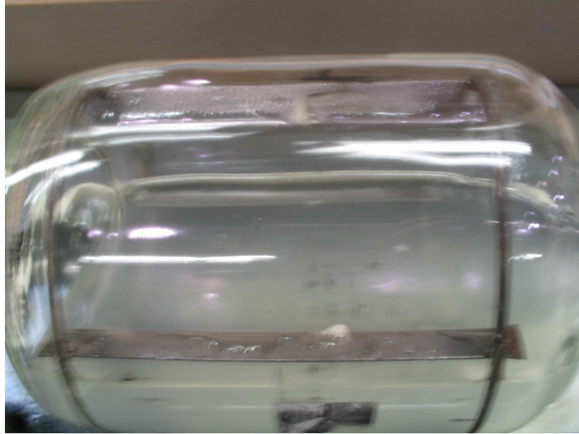
Figure 5.10: Mixed substrate particles clumped and stuck to the baffles in the baffled bioreactor (picture taken at 2 minutes after the start)
