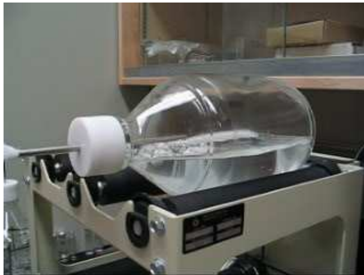
Figure 5.2: Naphthalene particles were sitting on the top of the aqueous phase in the control bioreactor (picture taken after 15 minutes from starting the roller apparatus).
