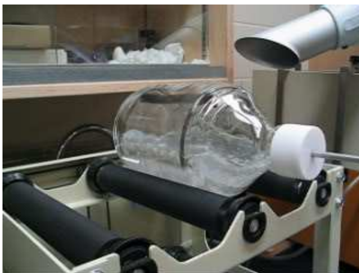
Figure 5.3: Naphthalene particles were completely mixed into the solution in the baffled bioreactor (picture taken after 15 minutes).
