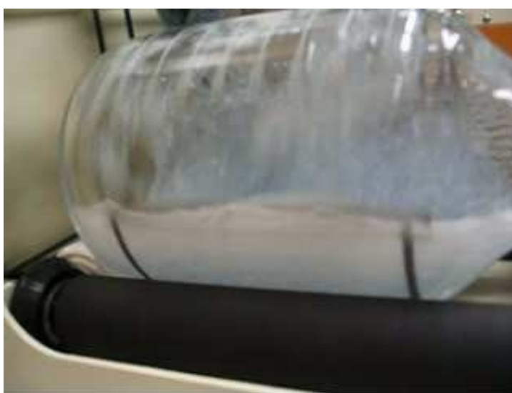
Figure 5.4: Mixing and crushing of naphthalene particles by the glass beads in the baffled BMB (picture taken after 15 minutes).
