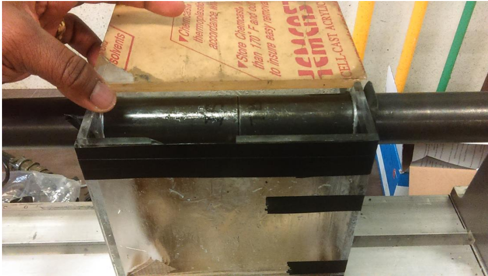
Fig. B.1 Position of the incident and transmitted bars the sample chamber during calibration
