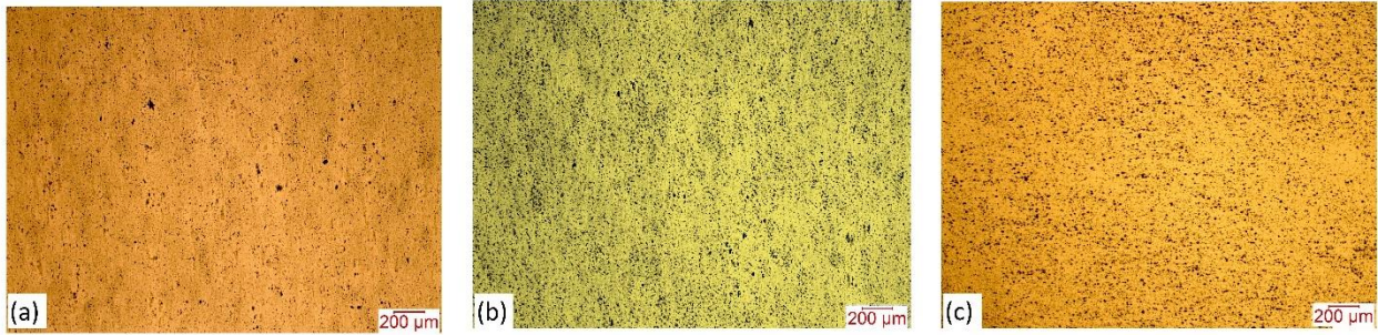
Fig. 4.8. Optical micrographs showing the distribution of second phase particles in the (a) AA 2024-T351, (b) AA 2624-T651 and (c) AA 2624-O alloy before mechanical loading.
