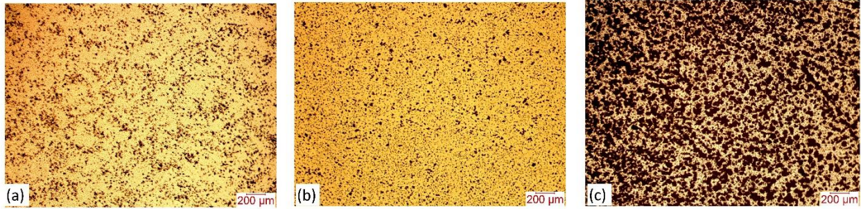
Fig. 4.2. Optical micrographs showing the distribution of second phase particles in the (a) AA 2017-T451, (b) AA 2017-T651 and (c) AA 2017-O alloy before mechanical loading.
