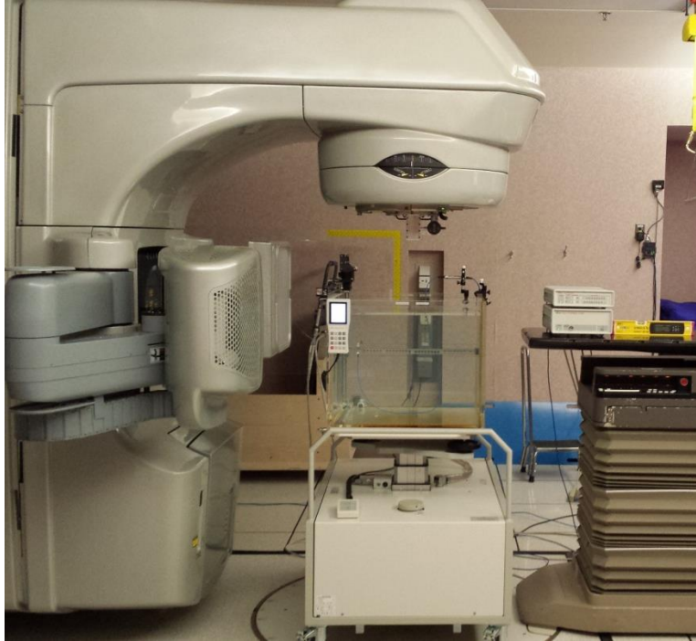
Figure 5.4. Linac 1 with the mini-beam collimator installed, the MP3 water phantom positioned, and the TANDEM electrometer unit connected to the detector.
