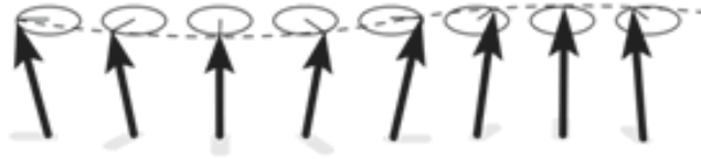
Figure 5.7: Conceptual drawing of a magnon propagating through a crystal. This figure was adapted from the material presented by Ref. 52.
