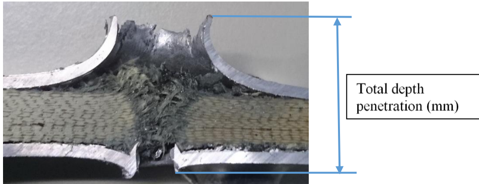
Fig. 5.5. Total depth penetration channel on the transverse section of the targets.
