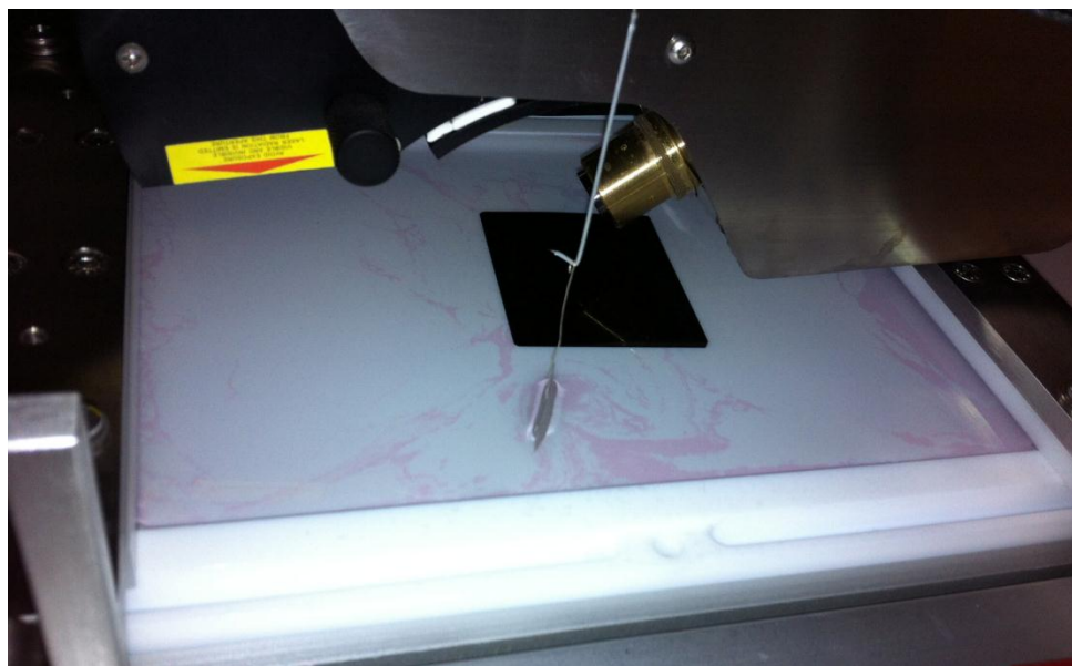
Figure 3-2. Photograph of the experimental apparatus and the air-water interface after ~ 60 minutes of UV illumination. The red PDA photoproduct is readily visible in the image.
