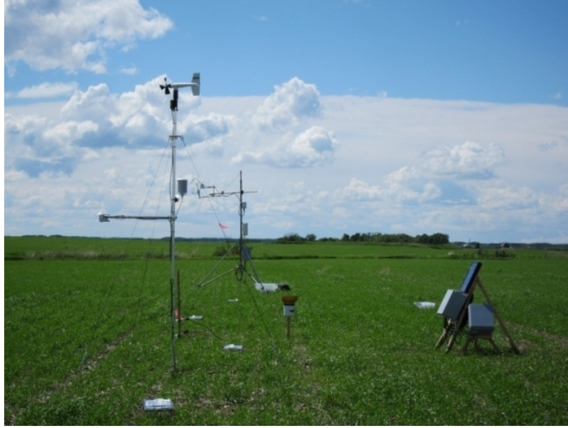
Fig. 3.2. Eddy covariance with all other instruments above soil ground
