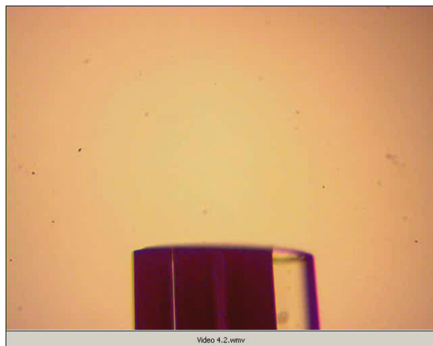
Video 4.2 Solution flow around a hot Bi microelectrode during the reduction of 50 mM methyl viologen in 0.2 M KCl. The electrode was heated with an alternating voltage of 13.4V_{\text{rms}} at 20 MHz (see Appendix E2 for individual frames).
