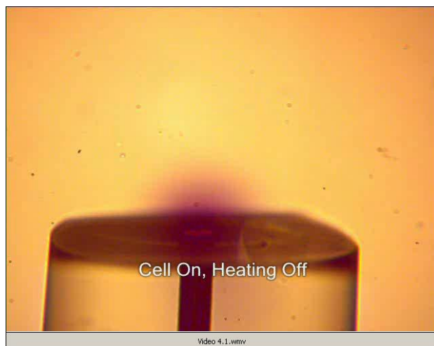
Video 4.1 Solution flow around a hot Pt microelectrode during the reduction of 50 mM methyl viologen in 0.2 M KCl. The electrode was heated with an alternating voltage of 13.4V_{\text{rms}} at 20 MHz (see Appendix E2 for individual frames).
