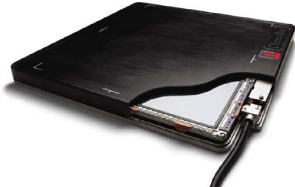
Figure 1.1: An image of a flat panel active matrix direct conversion X-ray image sensor [6].
