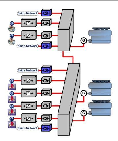
Figure 2.1: Conventional diesel-electric system (courtesy of E-MS)
