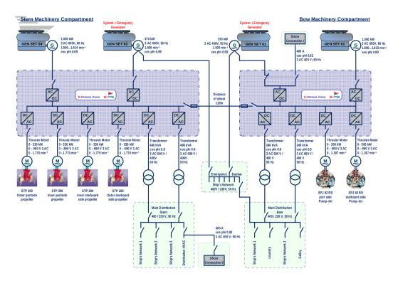
Figure 2.4: Network topology on the MS Viking Prestige (courtesy of E-MS)
