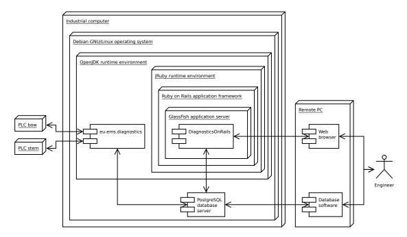
Figure 5.1: Deployment diagram of the diagnostic system on the MS Viking Prestige
