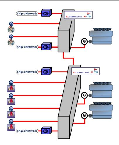
Figure 2.3: Diesel-electric system on the MS Viking Legend (courtesy of E-MS)
