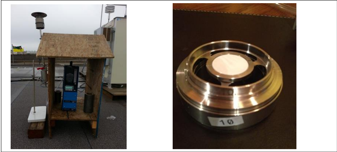
Figure 3-2. The Sampler and a Sample stage with filter.
