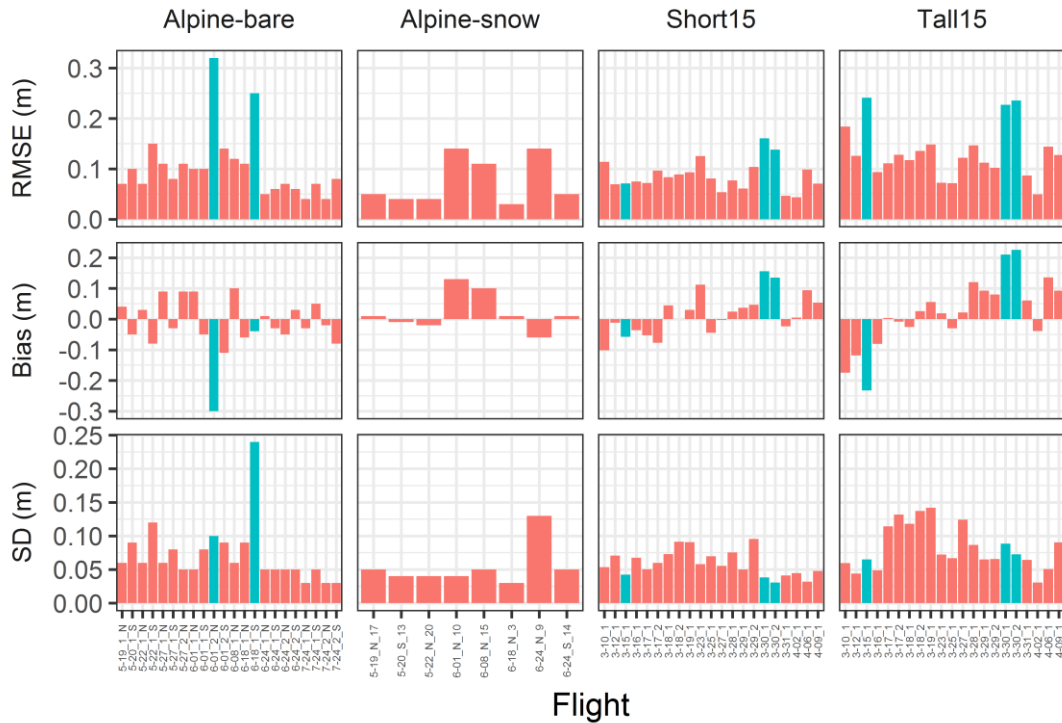
Figure 2.4: Root mean square error (RMSE, top row), Bias (middle row) and standard deviation (SD, bottom row) of DSMs with respect to surface over alpine-bare, alpine-snow, and short15 and tall15 stubble at prairie site, respectively. Blue bars highlight problematic flights and are excluded from summarization in Table 2.2. X-axis labels represent month-date-flight number of the day (to separate flights that occurred on the same day). Alpine-bare accuracies are separated into north or south areas, reflected with a _N or _S suffix. The last number in the alpine-snow x-axis label is the number of observations used to assess accuracy as the number of surface observations varied between 3 and 20.
