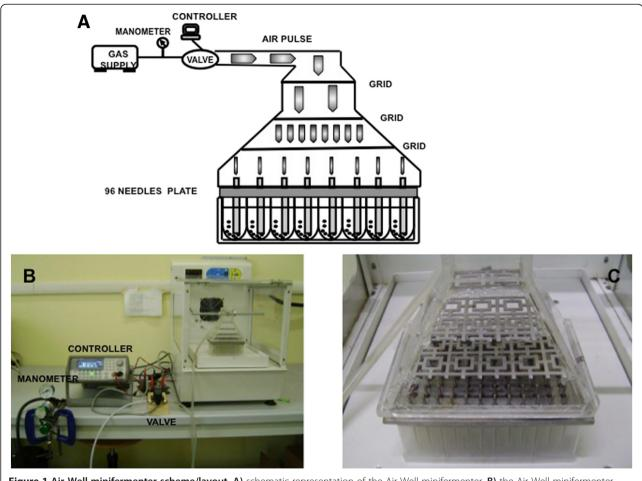
Figure 1 Air-Well minifermenter scheme/layout. A) schematic representation of the Air-Well minifermenter. B) the Air-Well minifermenter. C) Magnification of the Plexiglas bell with the grid used to equally split the air flux.
