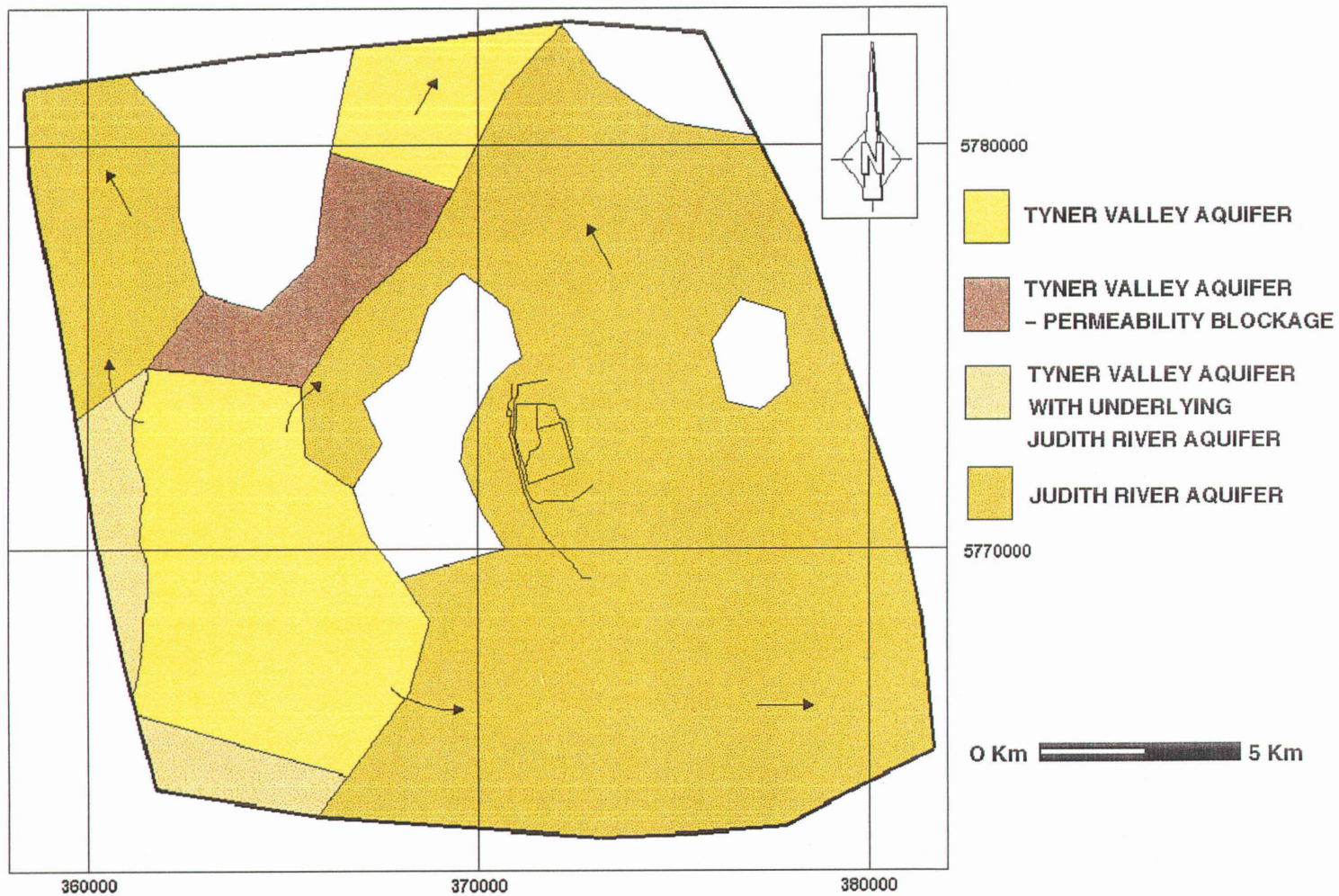
Figure 2.6 - Areal Extent and Direction of Groundwater Flow in the Tyner Valley Aquifer System
