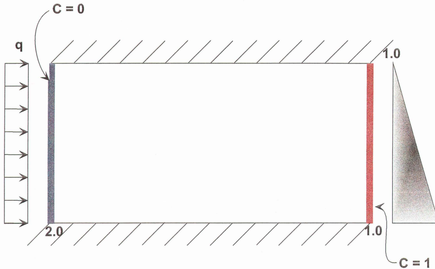
Figure A.1 - Problem domain and boundary conditions for the Henry (1964) seawater intrusion problem
