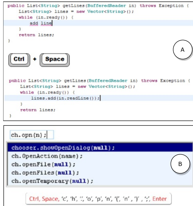
Figure 2.8: Examples of keyword-based code completion. The top figure (A) shows an example of code completion that translates input words into a valid expression (collected from Little and Miller [77]). The bottom figure (B) shows an example of abbreviated code completion (collected from Han et al. [40])
