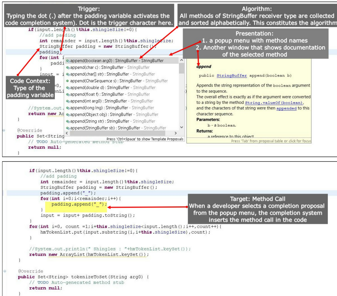
Figure 2.1: Five different components (trigger, algorithm, code context, presentation, and target) of a code completion system
