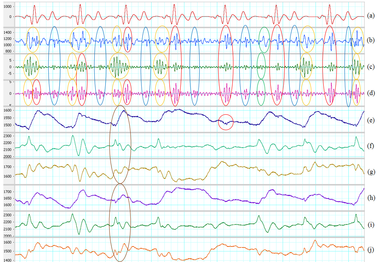
Figure 4.21 Two horizontal sensors with digital processing on walking motion. (a) Filtered ECG (5-20 Hz). (b) Filtered SCG with SUBTRACTOR ( subtraction ). (c) Filtered total acceleration . (d) Filtered z-axis acceleration . Red ovals indicate recognized systoles. Blue ovals indicate determined diastoles. Orange ovals show results of different response. Green ovals illustrate better noise suppression. (e) First sensor z-axis . Red circle indicates a small SCG signal. (f) First sensor y-axis . (g) First sensor x-axis . Brown oval indicates high-energy portion of walking. (h) Second sensor z-axis . (i) Second sensor y-axis . (j) Second sensor x-axis . Brown oval indicates high-energy portion of walking.
