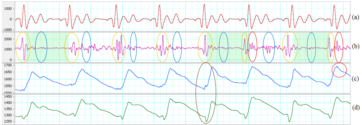
Figure 4.28 Two vertical sensors with AGC on walking motion. (a) Filtered ECG (5-20 Hz). (b) Filtered SCG (20-50 Hz). Orange ovals show results of different response and introduced noise. Red ovals indicate recognized systoles. Blue ovals indicate detected diastoles. Transparent green rectangles are periods with reduced gain after a detected saturation. (c) First sensor z-axis. Red circle indicates a small SCG signal. (d) Second sensor z-axis.
