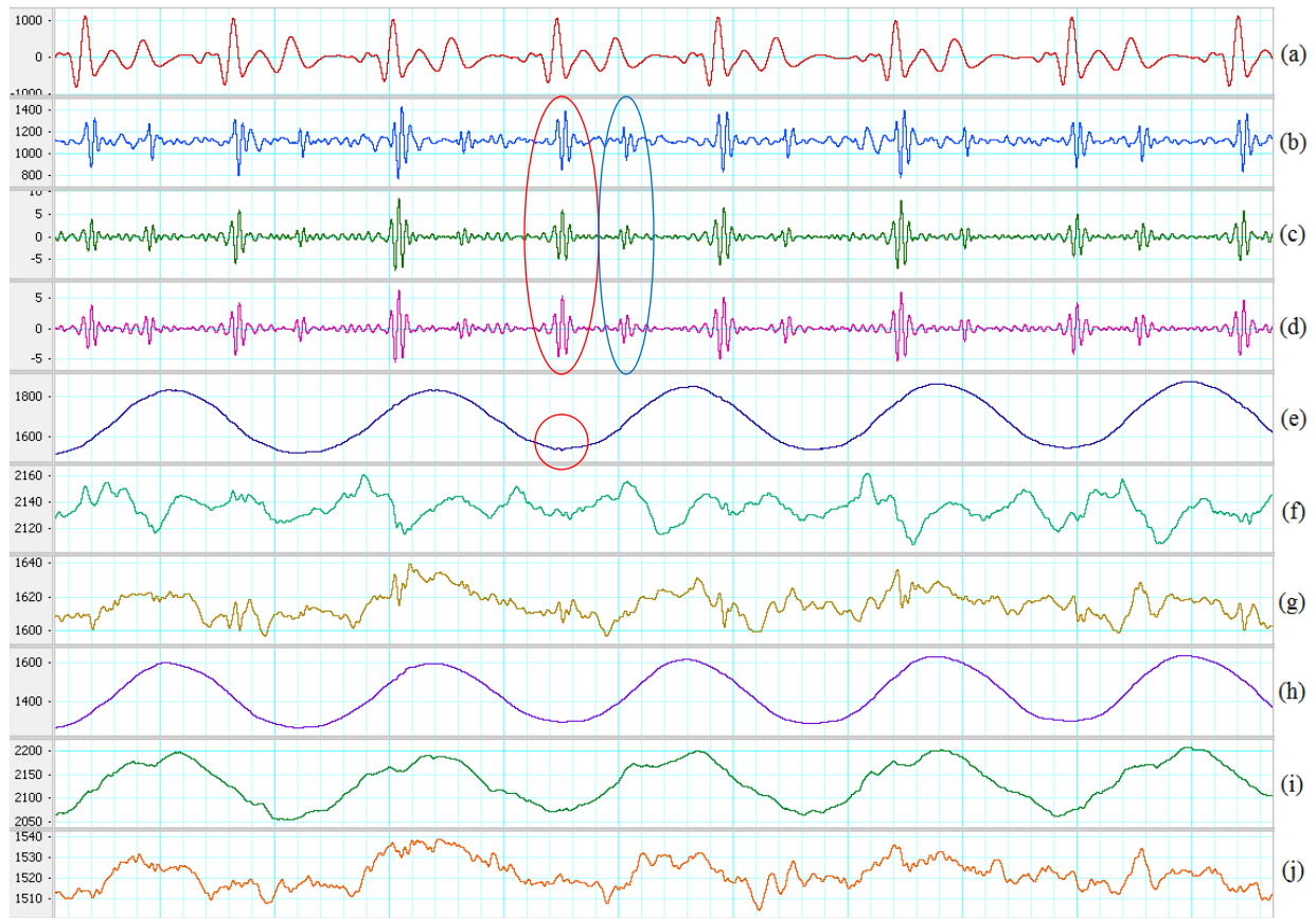
Figure 4.20 Two diagonal sensors with digital processing on gentle movement. (a) Filtered ECG (5-20 Hz). (b) Filtered SCG with SUBTRACTOR ( subtraction ). (c) Filtered total acceleration . (d) Filtered z-axis acceleration . Red oval indicates a recognized systole. Blue oval indicates a determined diastole. (e) First sensor z-axis . Red circle indicates a small SCG signal. (f) First sensor y-axis . (g) First sensor x-axis . (h) Second sensor z-axis . (i) Second sensor y-axis . (j) Second sensor x-axis .
