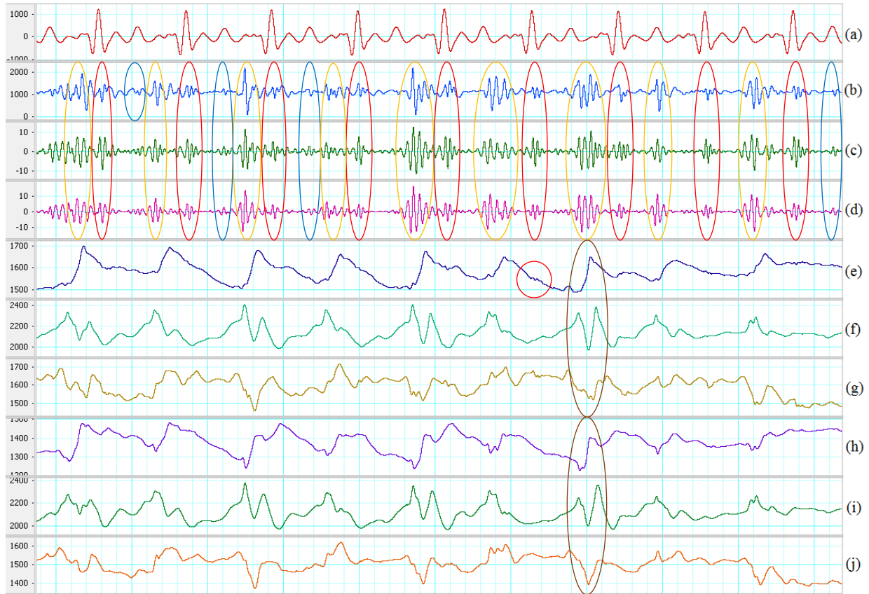
Figure 4.23 Two diagonal sensors with digital processing on walking motion. (a) Filtered ECG (5-20 Hz). (b) Filtered SCG with SUBTRACTOR ( subtraction ). (c) Filtered total acceleration . (d) Filtered z-axis acceleration . Red ovals indicate recognized systoles. Blue ovals indicate determined diastoles. Orange ovals show results of different response. (e) First sensor z-axis . Red circle indicates a small SCG signal. (f) First sensor y-axis . (g) First sensor x-axis . Brown oval indicates high-energy portion of walking. (h) Second sensor z-axis . (i) Second sensor y-axis . (j) Second sensor x-axis . Brown oval indicates high-energy portion of walking.
