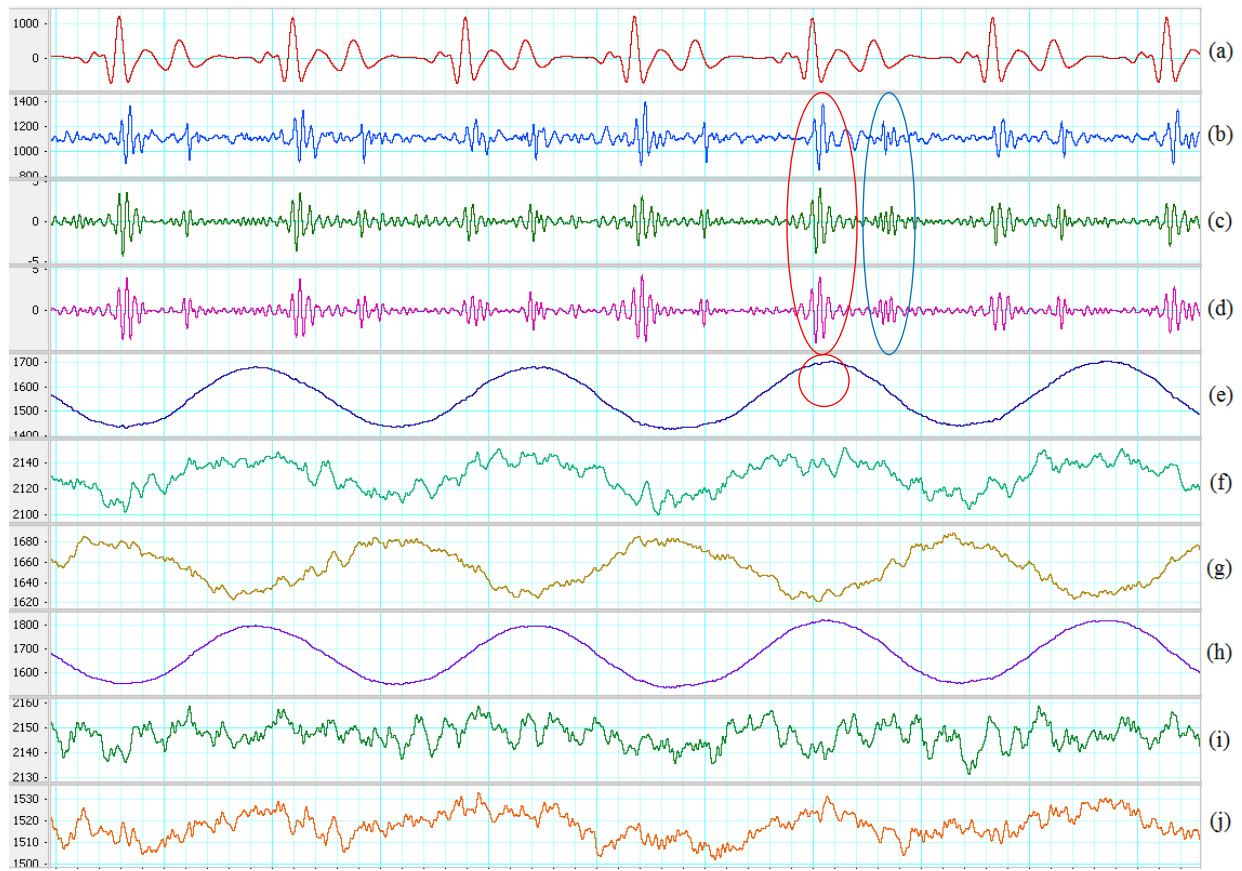
Figure 4.18 Two horizontal sensors with digital processing on gentle movement. (a) Filtered ECG (5-20 Hz). (b) Filtered SCG with SUBTRACTOR ( subtraction ). (c) Filtered total acceleration . (d) Filtered z-axis acceleration . Red oval indicates a recognized systole. Blue oval indicates a determined diastole. (e) First sensor z-axis . Red circle indicates a small SCG signal. (f) First sensor y-axis . (g) First sensor x-axis . (h) Second sensor z-axis . (i) Second sensor y-axis . (j) Second sensor x-axis .
