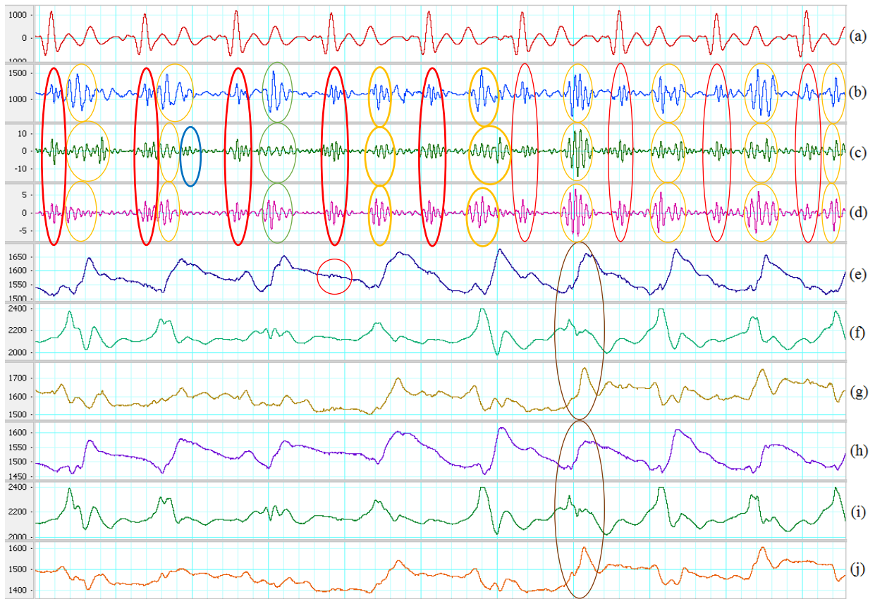
Figure 4.22 Two vertical sensors with digital processing on walking motion. (a) Filtered ECG (5-20 Hz). (b) Filtered SCG with SUBTRACTOR ( subtraction ). (c) Filtered total acceleration . (d) Filtered z-axis acceleration . Red ovals indicate recognized systoles. Blue ovals indicate determined diastoles. Orange ovals show results of different response. Green ovals illustrate better noise suppression. (e) First sensor z-axis . Red circle indicates a small SCG signal. (f) First sensor y-axis . (g) First sensor x-axis . Brown oval indicates high-energy portion of walking. (h) Second sensor z-axis . (i) Second sensor y-axis . (j) Second sensor x-axis . Brown oval indicates high-energy portion of walking.
