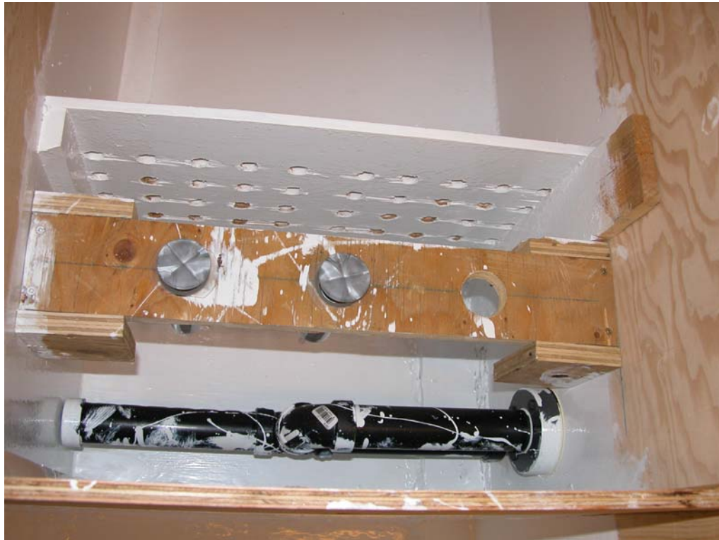
Figure 3.4 Diffuser and inlet chamber of the physical model.
