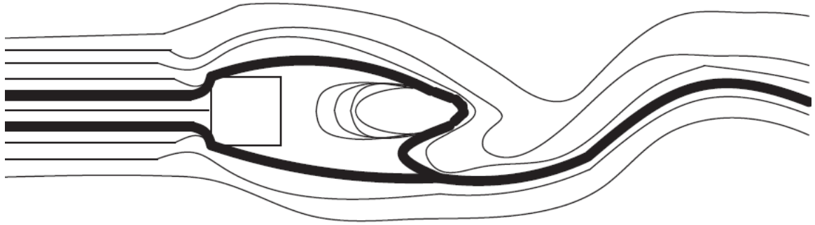
Figure 2.3 Flow pattern for a square cylinder at Reynolds number 150 (adapted from Okajima 1982).
