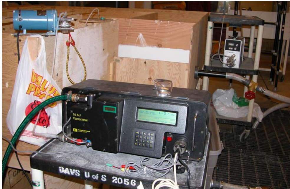
Figure 3.7 Fluorometer (Turner Designs Model 10) used in tracer tests.
