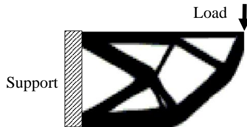
Figure 1-12 A structure design example based on continuum discretization
