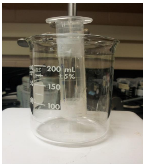
Figure A-2 The in-situ filtration device for roxarsone kinetic sampling
