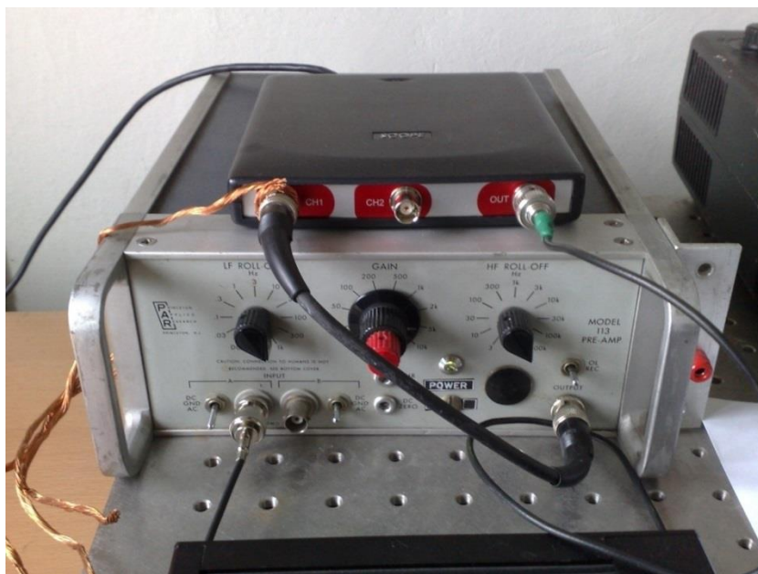
Figure 3:°The instruments used in experimental set-up with connections including digital oscilloscope (TiePie HS3) and power amplifier.
