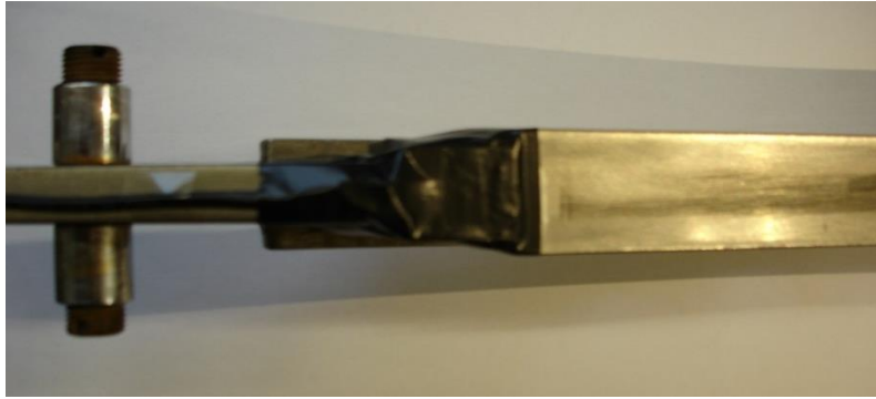
Figure 7: Mounting of the stationary (piezoelectric SAW) transducer at the far end of DC9 slat track during experiment.
