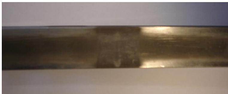
Figure 6:°Optical image of wear and corrosion (near center) on the surface of titanium built slat track of a DC9 aero-plane.
