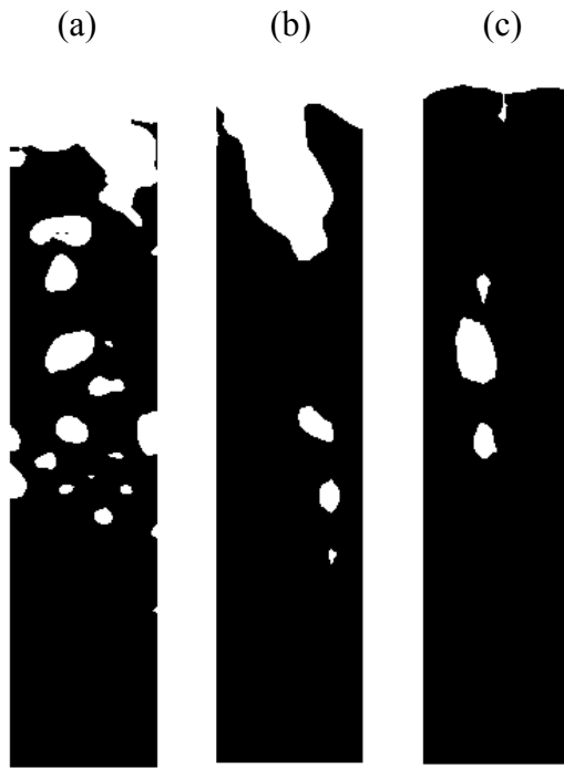
Figure 4.3c. Binary versions of the snapshots provided in Fig. 4.3b, a) 0.5 cm grid, b) 1 cm grid, c) 2 cm grid, the width of the images is 14 cm.
