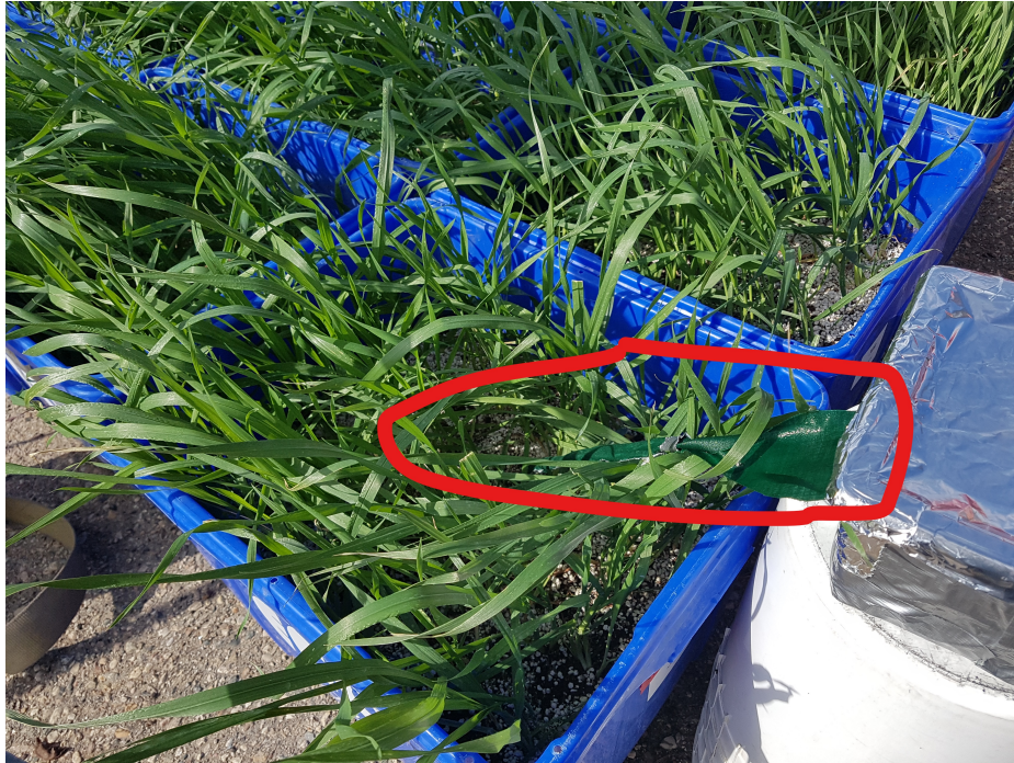
Figure 5.1: Wet reference in the spare tub of Stettler wheat circled in red. The water container and ribbon leading to the leaf are visible on the right.
