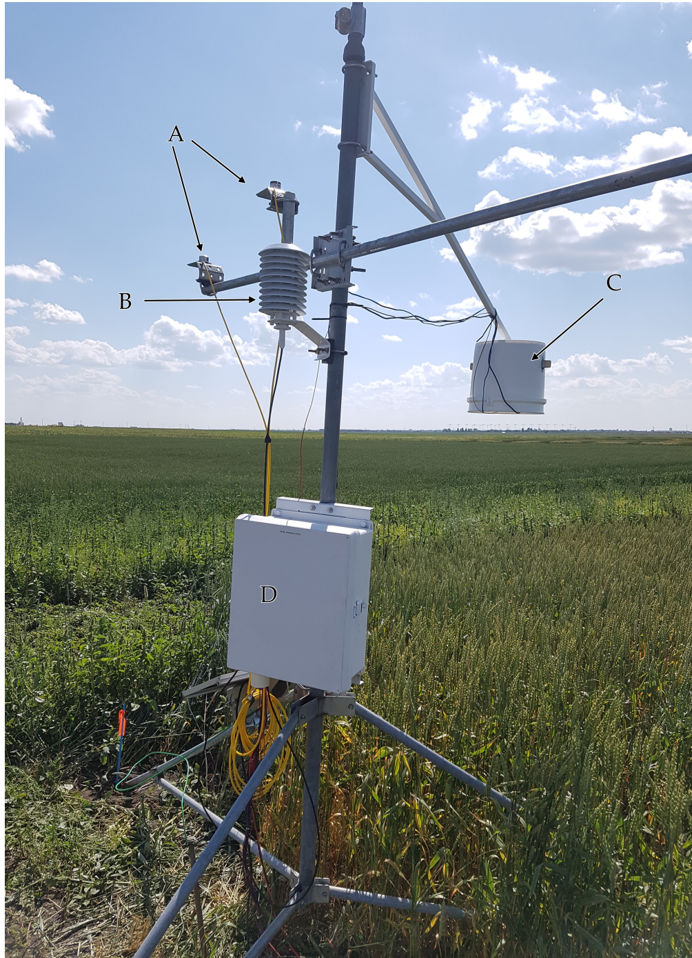
Figure 4.1: The weather station in field. A: pyranometers, B: ambient temperature and humidity sensor, C: thermal camera within a radiation shield, D: weatherproof cabinet with power supplies and the datalogger. Not shown: the wind speed sensor.
