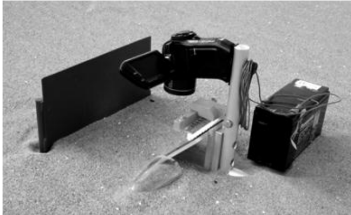
Figure 1: Setup used at the beach in Zingst, including a plate to shield the horizon, the stand with the mirror, the swiveling holder with the LED's and the high-speed camera. A plastic body for smoothing the air flow is fitted in front of the stand.
