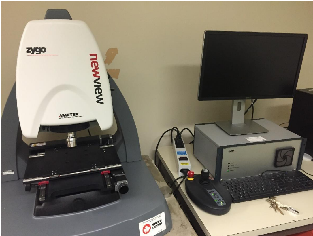
Figure 3-3. Zygo NewView 8000 optical profilometer
