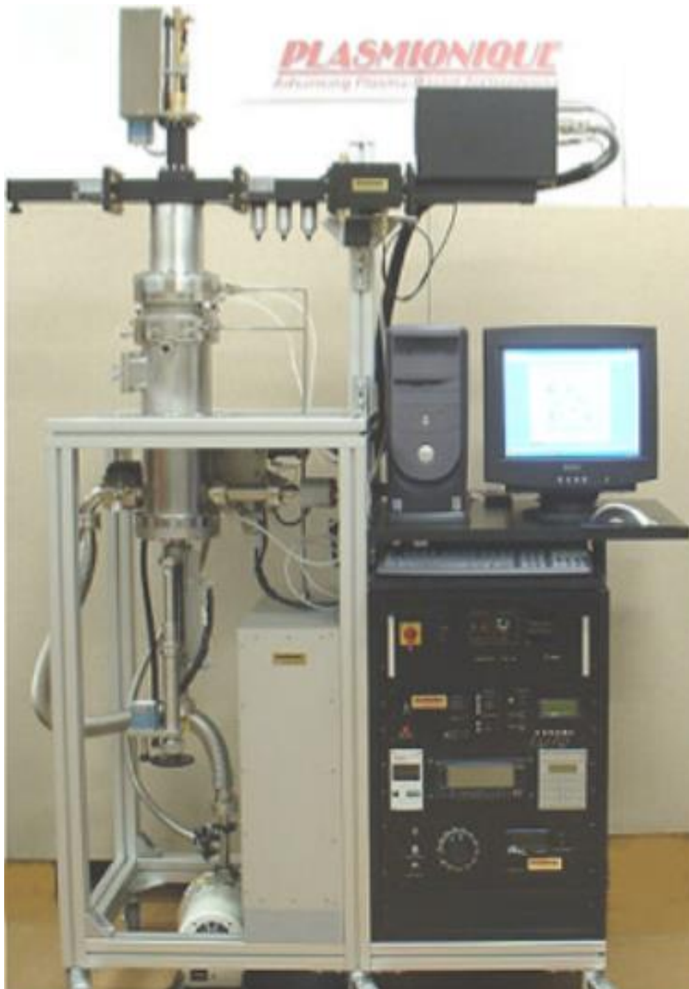
Figure 3-2. Microwave plasma enhanced chemical vapor deposition instrument (from Plasmionique)
