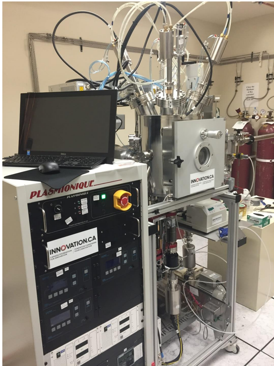
Figure 3-1. Magnetron sputtering instrument
