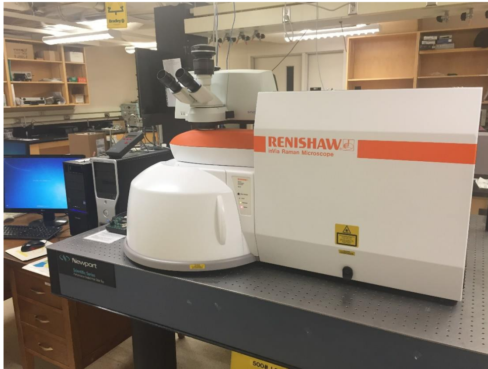
Figure 3-4. Renishaw 2000 Raman spectroscopy
