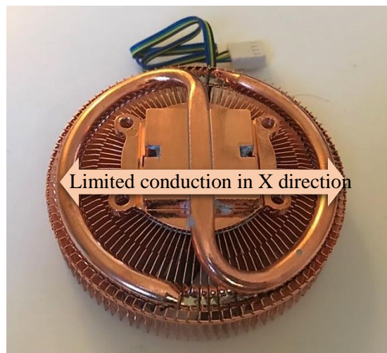
Figure 5-1. Heat pipes and thermal spreading resistance
