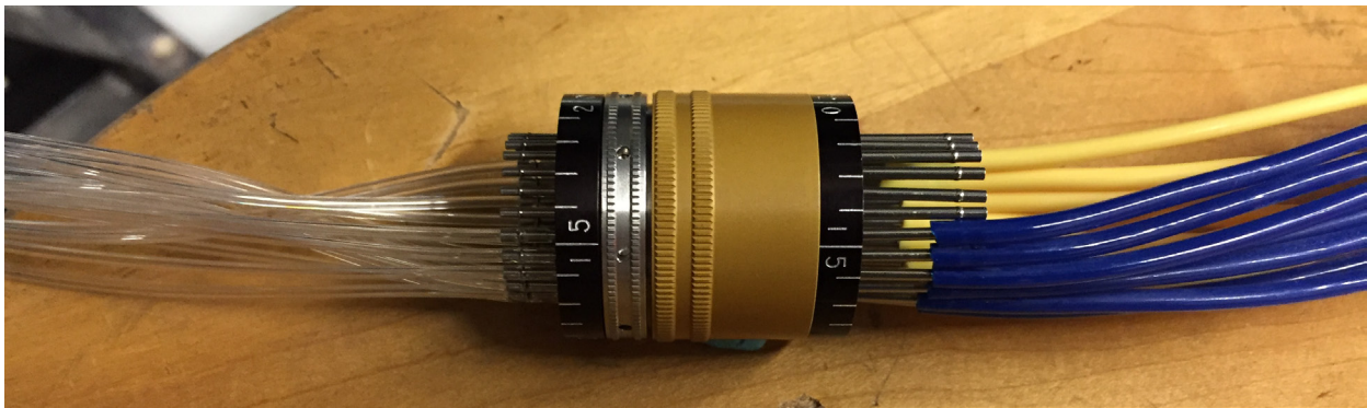
Figure 3.3: 24D round pneumatic connector from Scanivalve.
