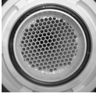
Figure 4.3. Photograph of the honeycomb flow straighteners placed before all of the orifice plates in the energy exchanger test facility (Erb, 2007).
