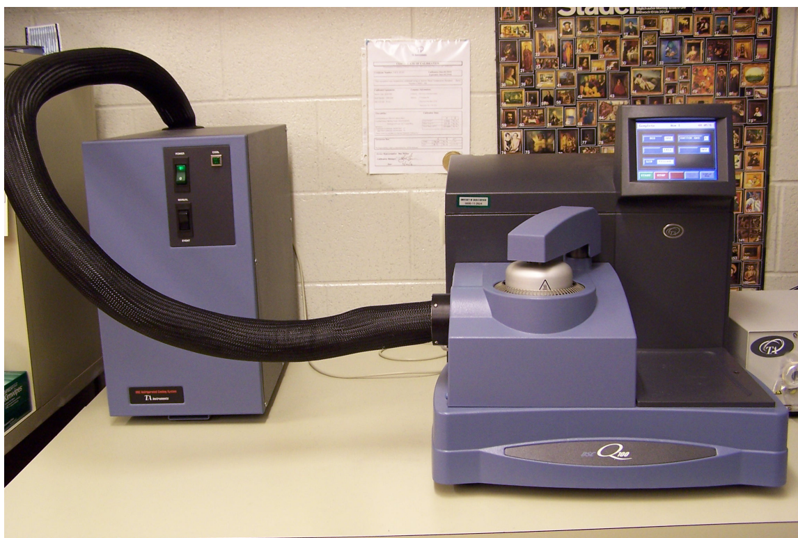
Figure 4.6 Model Q100, TA Instruments is a versatile research-grade DSC with capabilities to run modulated DSC experiments and built in TZERO™ technology.
