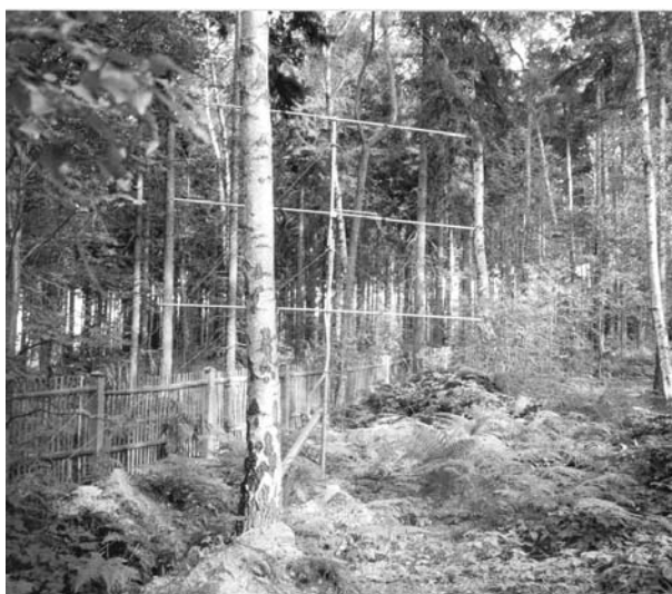
Figure 1: Left: Transmit antenna. In the foreground the trench to carry the feeder cable is still open. Right: Transmitter (right rack) and receiver unit (left rack) installed on a table.
