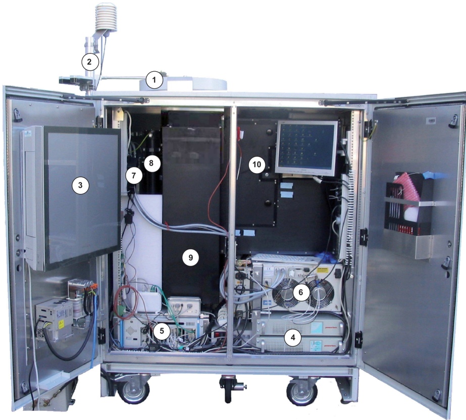
Figure 2.3: Polly XT cabinet with open doors: (1) roof cover, (2) sensors for outdoor temperature, air pressure and rain, (3) air condition, (4) uninterruptible power supply, (5) computer with data acquisition, (6) laser power supply, (7) laser head, (8) beam expander, (9) receiver telescope and (10) receiver with seven channels [Baars, 2012].
