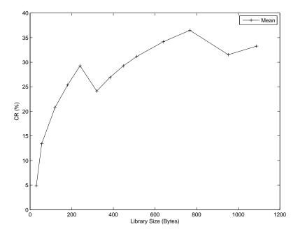
Figure 3.9: Effect of library size on mean CR for 20 endoscopic colour-scale images
