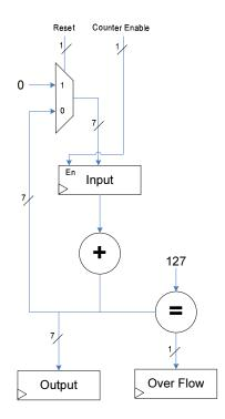
Figure 4.5: The architecture of the counter
