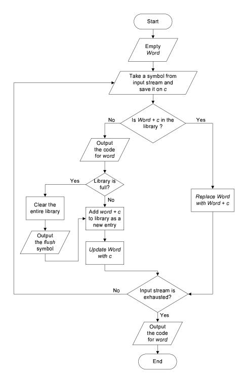
Figure 2.8: Flow chart of LZW–Flush algorithm
