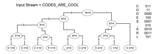
In [19], [21], the authors have proposed different hardware implementations of the Huffman algorithm. As Huffman method requires two passes, it is not suitable for real-
