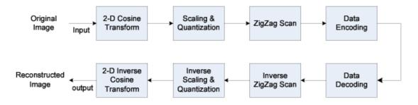
Figure 5.1: The image reconstruction process block diagram
