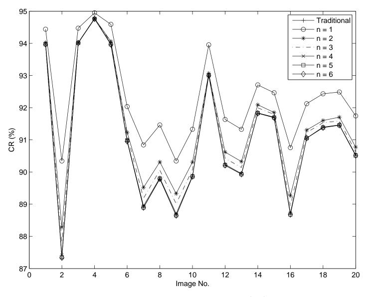
**Figure 3.5:** Effects of *n* on compression ratio (*CR*)
