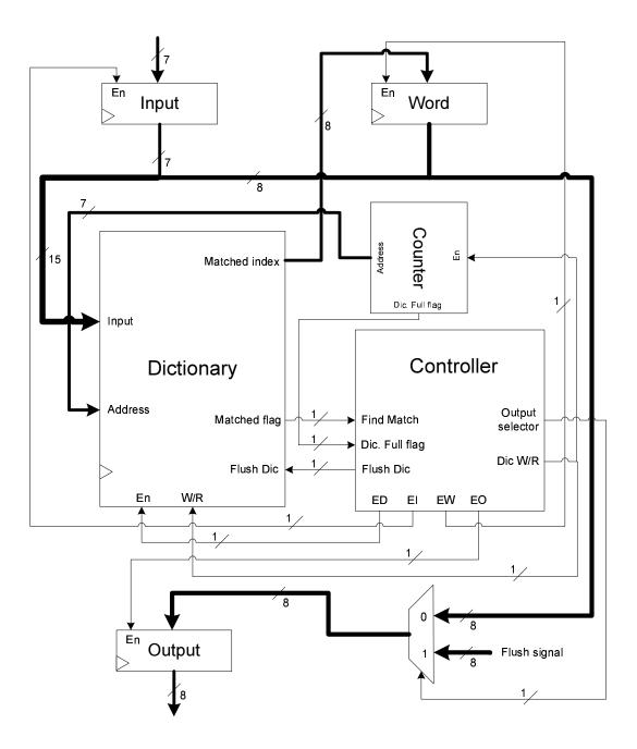
Figure 4.1: Hardware block diagram of the LZW–Flush encoder
