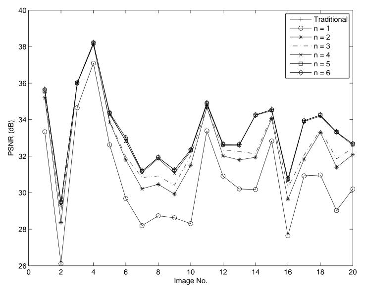
Figure 3.6: Effects of *n* on PSNR
