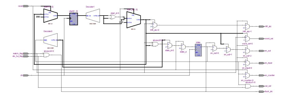
Figure 4.4: The architecture of the proposed controller
