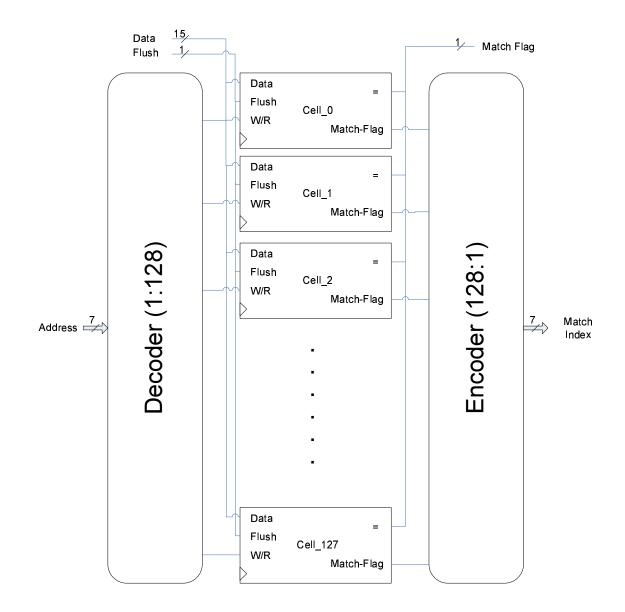
Figure 4.3: The architecture of entire proposed dictionary
