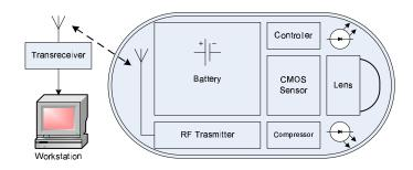
Figure 1.1: Block diagram of a typical endoscopic system [1]
