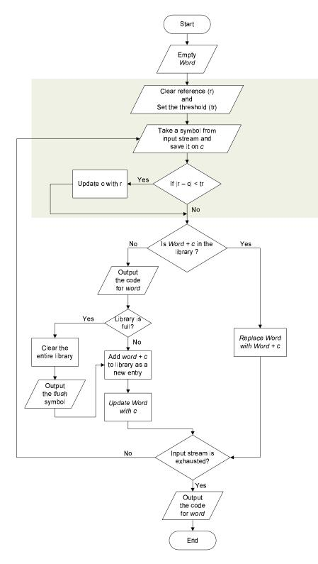
Figure 6.1: The lossy LZW–Flush algorithm flow chart
