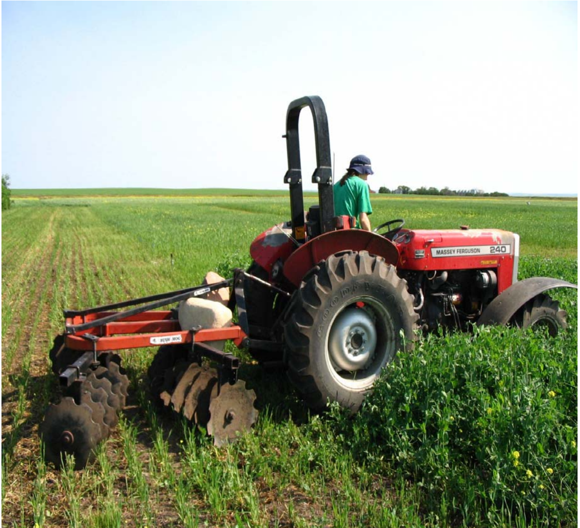
Figure 3-1 Small tractor equipped with a tandem disk incorporating green manure treatments nine weeks after seeding when the field pea was at full bloom at Vonda
