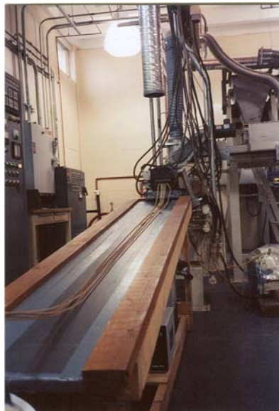
Figure 4.6 Perforated metal sheet on a platform with extruded strands being air-cooled.
