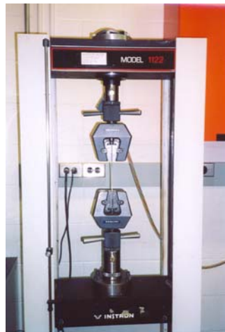
Figure 4.13 Instron reversible load cell (5 kN) (Instron, Canton, MA, USA) used to perform the tensile strength test.
