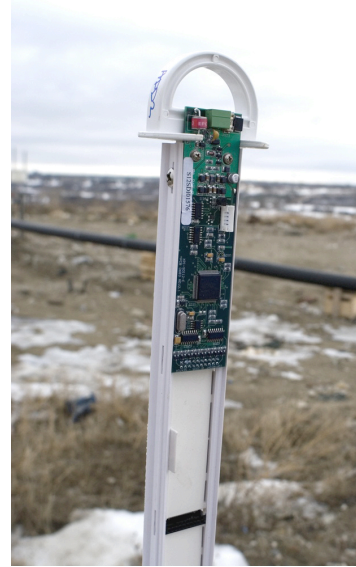
Figure 3.7 - SDI-12 circuit board, ES top handle and sensor rail.
