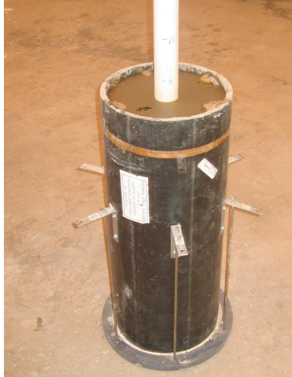
Figure 3.2 - Lab apparatus for compaction and testing of moisture content in MSW, pictured here in a saturated condition at the end of a trial. The vessel in this photograph is 0.75m tall.
