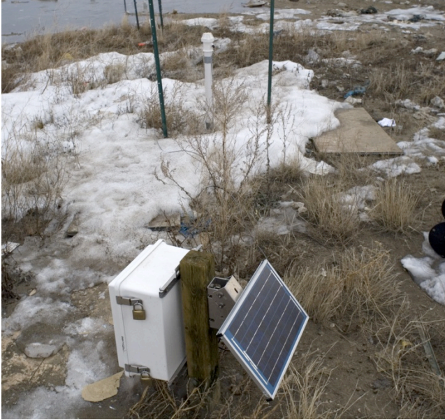
Figure 3.6 - Logging station (foreground) and ES probe (background).
