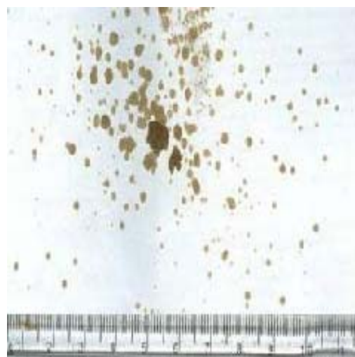
d: Spray with mixture of water and glycerol
