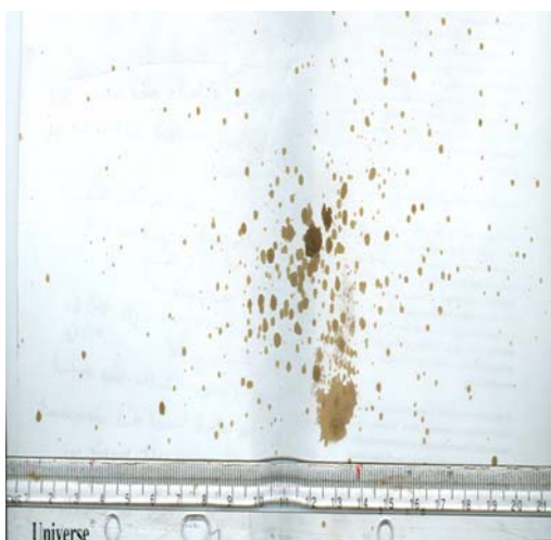
c: Spray with 70mL/min
